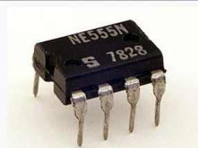
Signetics NE555 in 8-pin DIP package
